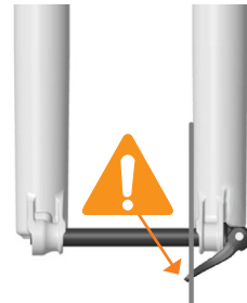
INCORRECTLY INSTALLED AXLE
